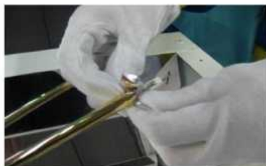
5. OPEN THE TWO METAL FLAPS POSITIONED ON THE EXTREMITIES OF THE BULB TO BE REPLACED AND, ON THE NEW BULB, RE-POSITION THE FLAPS, AS BEFORE.
