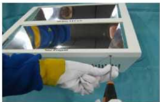
1. UNSCREW THE SCREWS HOLDING THE FRAME.
