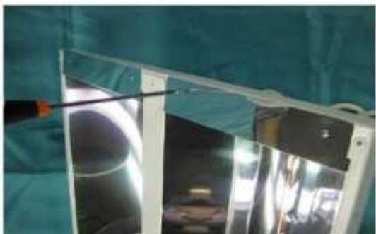
2. UNSCREW THE FOUR (4) SCREWS FASTENING THE SIDE COVERS OF THE REFLECTOR. REMOVE THE COVERS.
